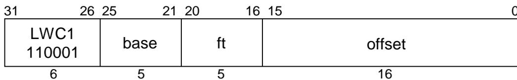
**MIPS I****Format:** LWC1 ft, offset (base)**Purpose:** To load a word from memory to an FPR.**Description:**  $ft \leftarrow \text{memory}[\text{base}+\text{offset}]$
