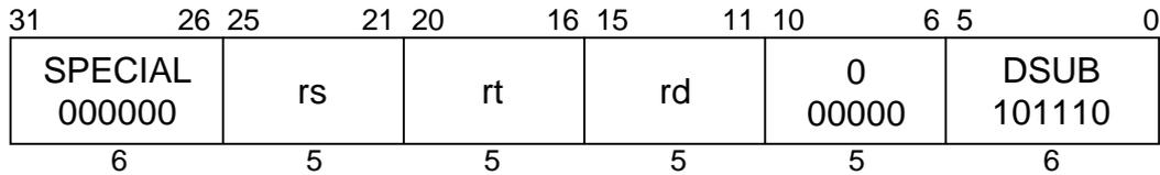
**MIPS III****Format:** DSUB rd, rs, rt**Purpose:** To subtract 64-bit integers; trap if overflow.**Description:**  $rd \leftarrow rs - rt$
