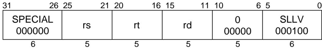
**MIPS I****Format:** SLLV rd, rt, rs**Purpose:** To left shift a word by a variable number of bits.**Description:**  $rd \leftarrow rt \ll rs$
