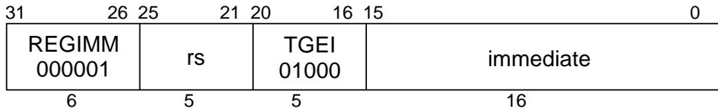
**MIPS II****Format:** TGEI rs, immediate**Purpose:** To compare a GPR to a constant and do a conditional Trap.**Description:** if ( $rs \geq \text{immediate}$ ) then Trap
