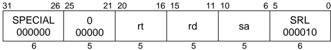
**MIPS I****Format:** SRL rd, rt, sa**Purpose:** To logical right shift a word by a fixed number of bits.**Description:**  $rd \leftarrow rt \gg sa$  (logical)
