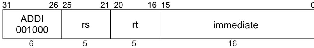
**MIPS I****Format:** ADDI *rt*, *rs*, *immediate***Purpose:** To add a constant to a 32-bit integer. If overflow occurs, then trap.**Description:**  $rt \leftarrow rs + \text{immediate}$
