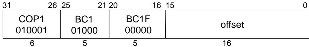
**MIPS I****Format:** BC1F offset**Purpose:** To test an FP condition code and do a PC-relative conditional branch.**Description:** if (C = 0) then branch where C is FCR31<sub>23</sub>
