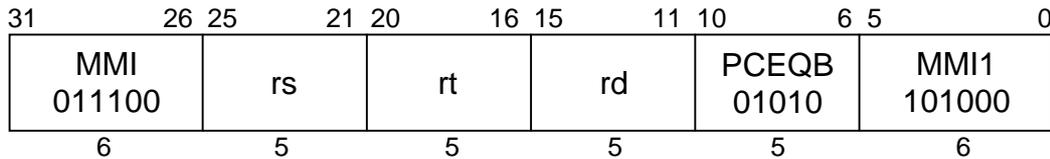
**C790****Format:** PCEQB rd, rs, rt**Purpose:** To record the result of 16 equality comparisons in parallel.**Description:**  $rd \leftarrow (rs = rt)$
