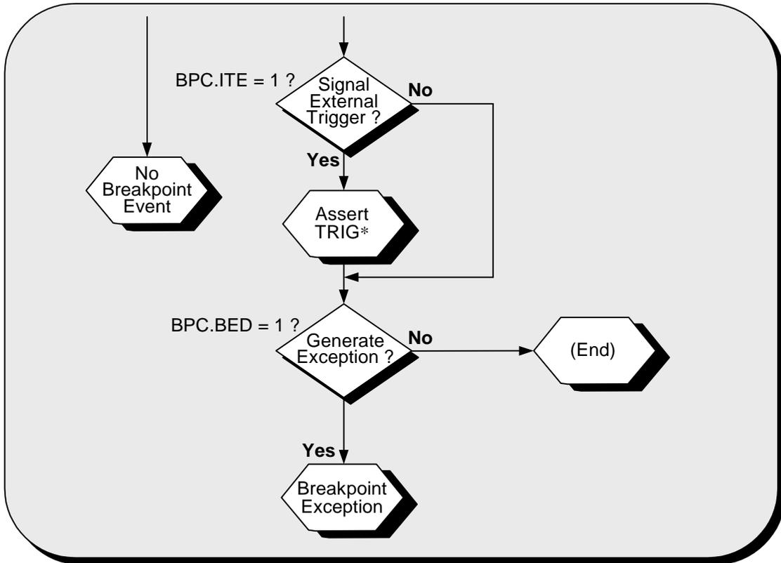
Figure 13-10. Hardware Breakpoint detection flow (IAB) (2/2)
