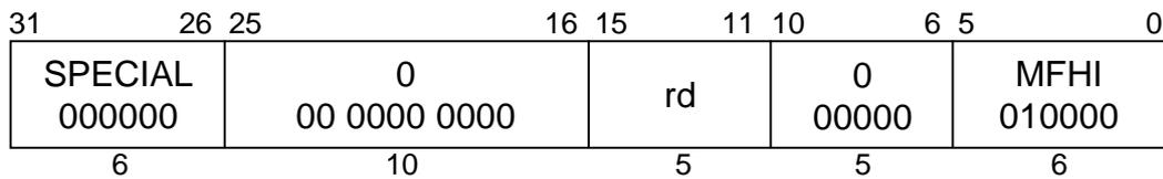
**MIPS I****Format:** MFHI rd**Purpose:** To copy the special purpose HI register to a GPR.**Description:** rd ← HI
