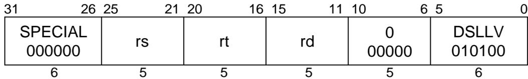
**MIPS III****Format:** DSLLV rd, rt, rs**Purpose:** To left shift a doubleword by a variable number of bits.**Description:**  $rd \leftarrow rt \ll rs$
