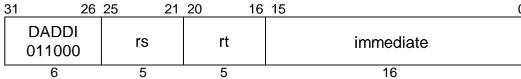
**MIPS III****Format:** DADDI rt, rs, immediate**Purpose:** To add a constant to a 64-bit integer. If overflow occurs, then trap.**Description:**  $rt \leftarrow rs + \text{immediate}$
