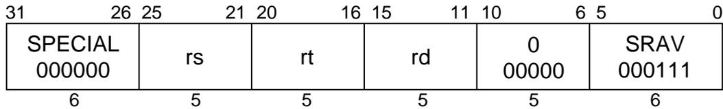
**MIPS I****Format:** SRAV rd, rt, rs**Purpose:** To arithmetic right shift a word by a variable number of bits.**Description:**  $rd \leftarrow rt \gg rs$  (arithmetic)
