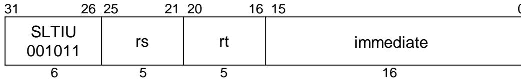
**MIPS I****Format:** SLTIU rt, rs, immediate**Purpose:** To record the result of an unsigned less-than comparison with a constant.**Description:**  $rt \leftarrow (rs < \text{immediate})$
