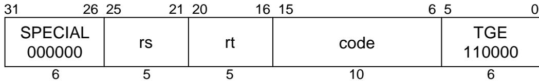
**MIPS II****Format:** TGE rs, rt**Purpose:** To compare GPRs and do a conditional Trap.**Description:** if ( $rs \geq rt$ ) then Trap
