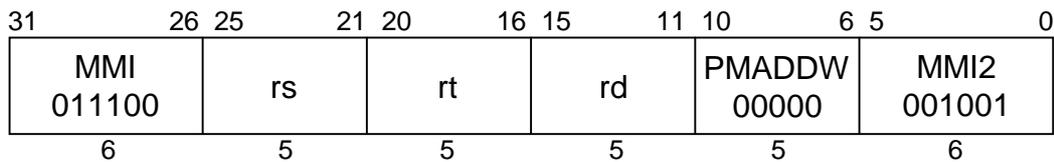
**C790****Format:** PMADDW rd, rs, rt**Purpose:** To multiply 2 pairs of 32-bit signed integers and accumulate in parallel.**Description:** (rd, HI, LO) ← (HI, LO) + rs × rt
