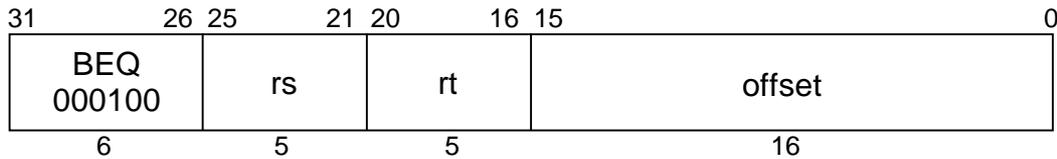
**MIPS I****Format:** BEQ rs, rt, offset**Purpose:** To compare GPRs then do a PC-relative conditional branch.**Description:** if (rs = rt) then branch
