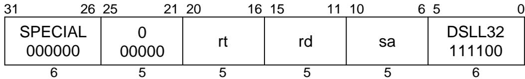
**MIPS III****Format:** DSLL32 rd, rt, sa**Purpose:** To left shift a doubleword by a fixed amount — 32 to 63 bits.**Description:**  $rd \leftarrow rt \ll (sa + 32)$
