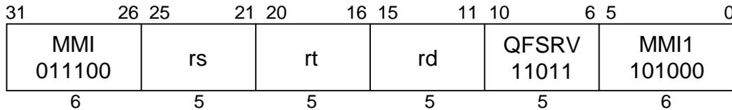
**C790****Format:** QFSRV rd, rs, rt**Purpose:** To right shift a quadword by a variable number of bits.**Description:**  $rd \leftarrow (rs, rt) \gg SA$
