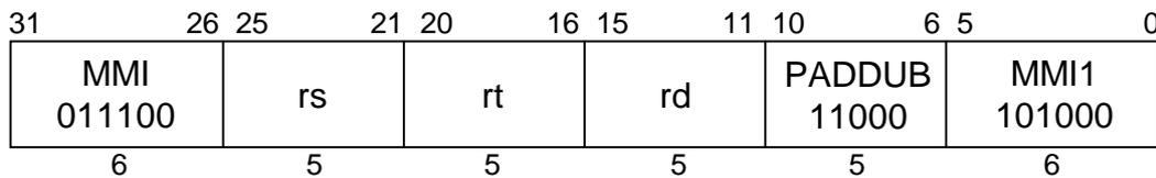
**C790****Format:** PADDUB rd, rs, rt**Purpose:** To add 16 pairs of 8-bit unsigned integers with saturation in parallel.**Description:**  $rd \leftarrow rs + rt$
