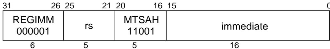
**C790****Format:** M TSAH rs, immediate**Purpose:** To copy a GPR to the shift amount register SA.**Description:**  $SA \leftarrow (rs \text{ xor } \text{immediate}) \times 16$
