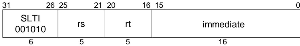
**MIPS I****Format:** SLTI *rt*, *rs*, *immediate***Purpose:** To record the result of a less-than comparison with a constant.**Description:**  $rt \leftarrow (rs < immediate)$
