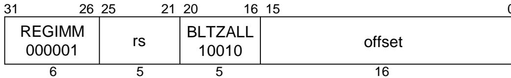
**MIPS II****Format:** BLTZALL rs, offset**Purpose:** To test a GPR then do a PC-relative conditional procedure call; execute the delay slot only if the branch is taken.**Description:** if (rs < 0) then procedure\_call\_likely
