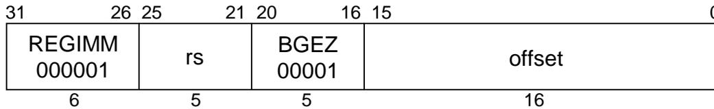
**MIPS I****Format:** BGEZ rs, offset**Purpose:** To test a GPR then do a PC-relative conditional branch.**Description:** if ( $rs \geq 0$ ) then branch
