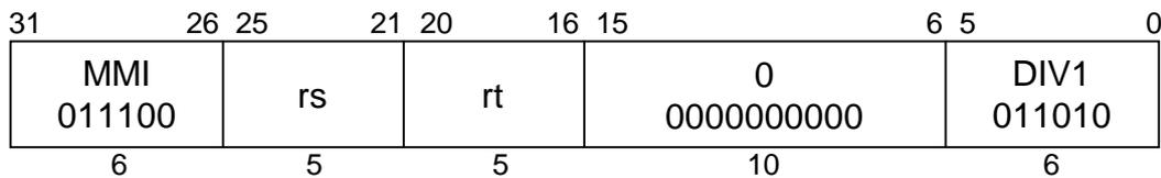
**C790****Format:** DIV1 rs, rt**Purpose:** To divide 32-bit signed integers using pipeline 1.**Description:** (LO1, HI1) ← rs / rt
