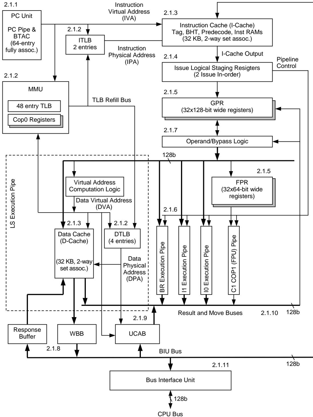
Figure 2-1. C790 Block Diagram
