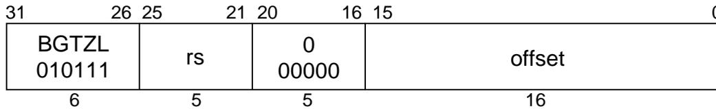
**MIPS II****Format:** BGTZL rs, offset**Purpose:** To test a GPR then do a PC-relative conditional branch; execute the delay slot only if the branch is taken.**Description:** if (rs > 0) then branch\_likely
