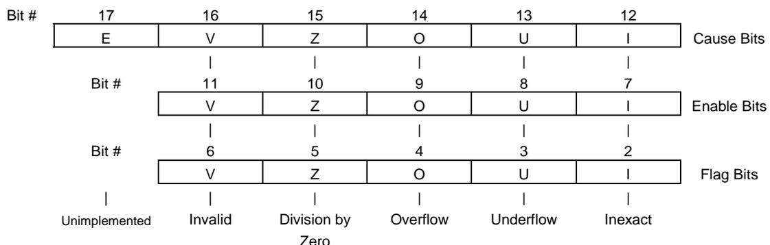
Figure 11-1. Control/Status Register Exception/Flag/Trap/Enable Bits
