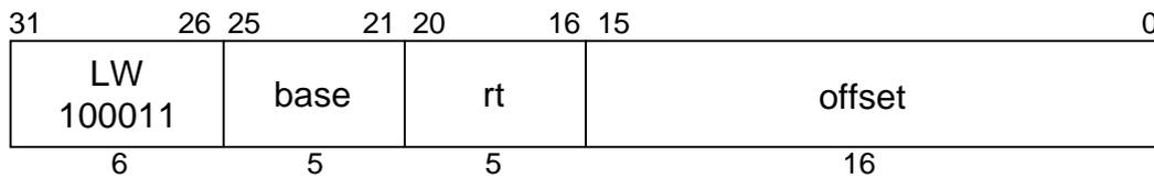
**MIPS I****Format:** LW *rt*, *offset* (*base*)**Purpose:** To load a word from memory as a signed value.**Description:**  $rt \leftarrow \text{memory}[\text{base} + \text{offset}]$
