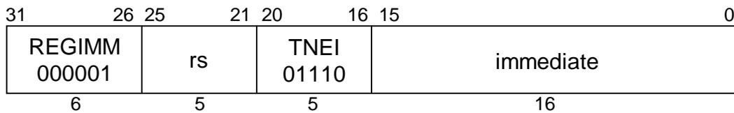
**MIPS II****Format:** TNEI rs, immediate**Purpose:** To compare a GPR to a constant and do a conditional Trap.**Description:** if (rs  $\neq$  immediate) then Trap
