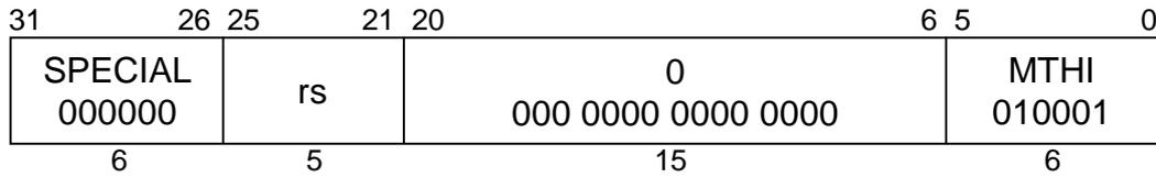
**MIPS I****Format:** MTHI rs**Purpose:** To copy a GPR to the special purpose HI register.**Description:** HI ← rs
