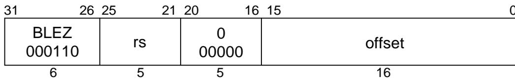
**MIPS I****Format:** BLEZ rs, offset**Purpose:** To test a GPR then do a PC-relative conditional branch.**Description:** if ( $rs \leq 0$ ) then branch
