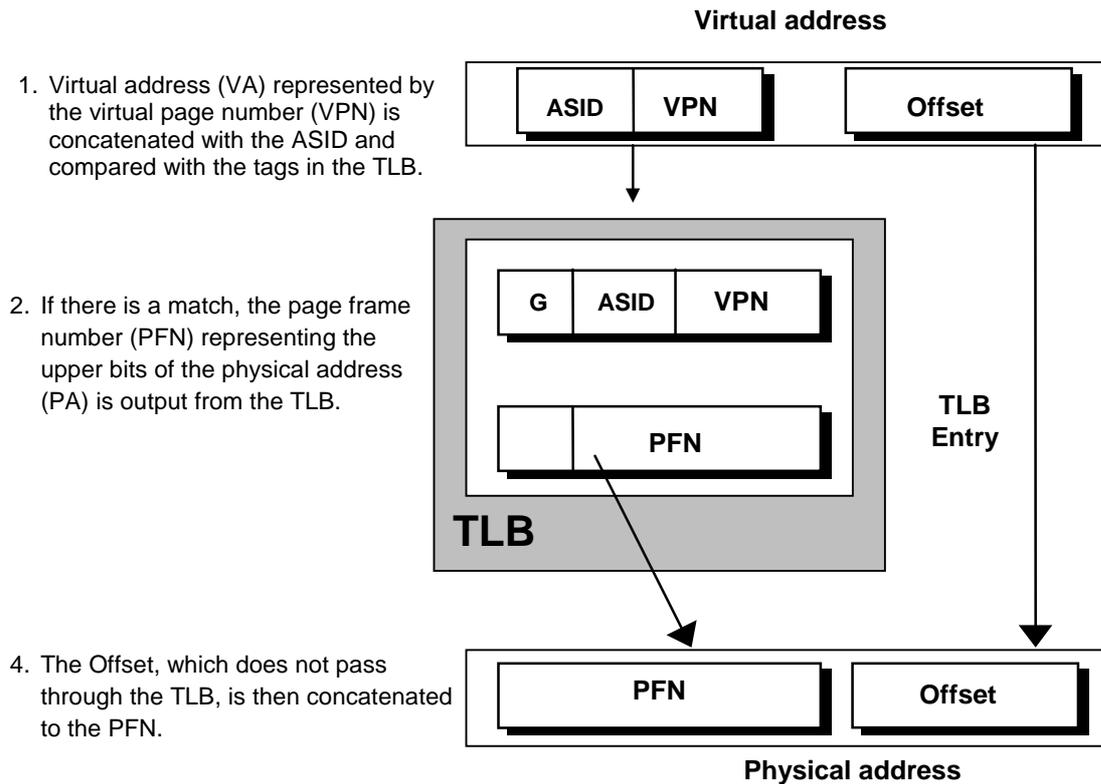
Figure 6-1. Overview of a Virtual-to-Physical Address Translation
