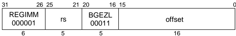
**MIPS II****Format:** BGEZL rs, offset**Purpose:** To test a GPR then do a PC-relative conditional branch; execute the delay slot only if the branch is taken.**Description:** if ( $rs \geq 0$ ) then branch\_likely
