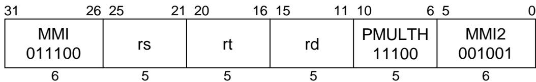
**C790****Format:** PMULTH rd, rs, rt**Purpose:** To multiply 8 pairs of 16-bit signed integers in parallel.**Description:** (rd, LO, HI)  $\leftarrow$  rs  $\times$  rt
