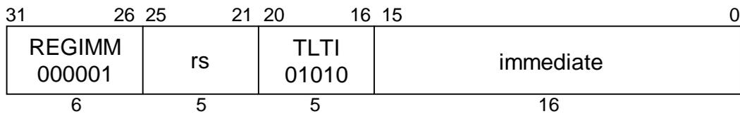
**MIPS II****Format:** TLTI rs, immediate**Purpose:** To compare a GPR to a constant and do a conditional Trap.**Description:** if (rs < immediate) then Trap
