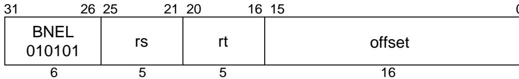
**MIPS II****Format:** BNEL rs, rt, offset**Purpose:** To compare GPRs then do a PC-relative conditional branch; execute the delay slot only if the branch is taken.**Description:** if ( $rs \neq rt$ ) then branch\_likely
