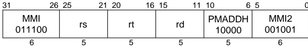
**C790****Format:** PMADDH rd, rs, rt**Purpose:** To multiply 8 pairs of 16-bit signed integers and accumulate, in parallel.**Description:** (rd, HI, LO) ← (HI, LO) + rs × rt
