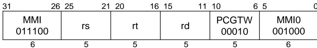
**C790****Format:** PCGTW rd, rs, rt**Purpose:** To record the results of 4 greater-than comparisons in parallel.**Description:**  $rd \leftarrow (rs > rt)$
