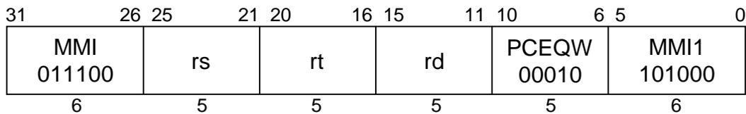
**C790****Format:** PCEQW rd, rs, rt**Purpose:** To record the result of 4 equality comparisons in parallel.**Description:**  $rd \leftarrow (rs = rt)$
