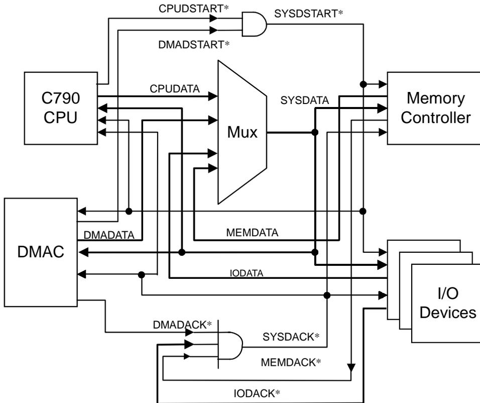
Figure 8-3. CPU Bus Data Path Connections in System
