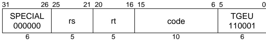
**MIPS II****Format:** TGEU rs, rt**Purpose:** To compare GPRs and do a conditional Trap.**Description:** if ( $rs \geq rt$ ) then Trap
