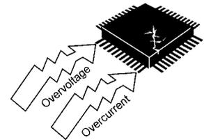
If the voltage or current on any pin exceeds the absolute maximum rating, the device's internal circuitry can become degraded. In the worst case, heat generated in internal circuitry can fuse wiring or cause the semiconductor chip to break down.
