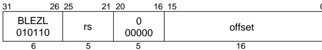
**MIPS II****Format:** BLEZL rs, offset**Purpose:** To test a GPR then do a PC-relative conditional branch; execute the delay slot only if the branch is taken.**Description:** if ( $rs \leq 0$ ) then branch\_likely
