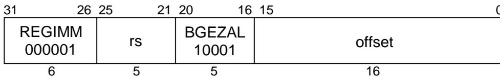
**MIPS I****Format:** BGEZAL rs, offset**Purpose:** To test a GPR then do a PC-relative conditional procedure call.**Description:** if ( $rs \geq 0$ ) then procedure\_call
