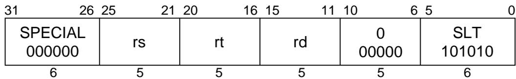
**MIPS I****Format:** SLT rd, rs, rt**Purpose:** To record the result of a less-than comparison.**Description:**  $rd \leftarrow (rs < rt)$
