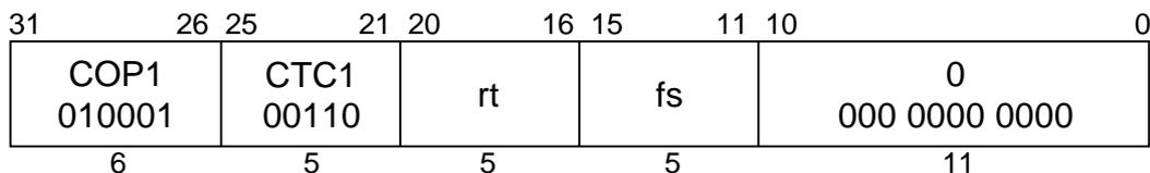
**MIPS I****Format:** CTC1 rt, fs**Purpose:** To copy a word from a GPR to an FPU control register.**Description:** FP\_Control[fs] ← rt
