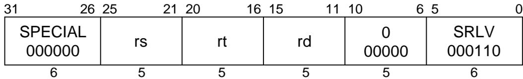
**MIPS I****Format:** SRLV rd, rt, rs**Purpose:** To logical right shift a word by a variable number of bits.**Descriptions:**  $rd \leftarrow rt \gg rs$  (logical)
