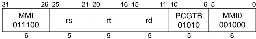
**C790****Format:** PCGTB rd, rs, rt**Purpose:** To record the result of 16 greater-than comparisons in parallel.**Description:**  $rd \leftarrow (rs > rt)$
