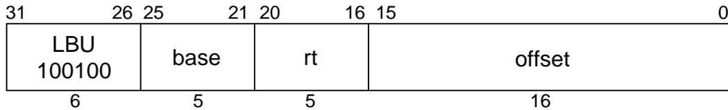
**MIPS I****Format:** LBU *rt*, *offset* (*base*)**Purpose:** To load a byte from memory as an unsigned value.**Description:**  $rt \leftarrow \text{memory}[\text{base} + \text{offset}]$
