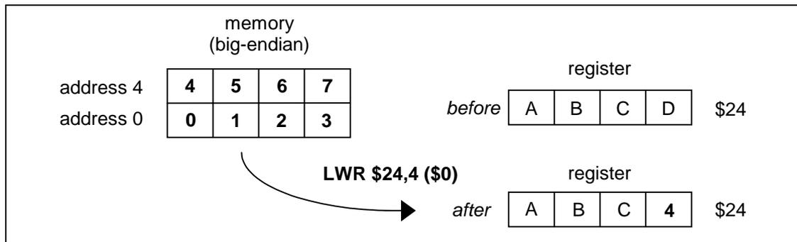
The contents of GPR *rt* are internally bypassed within the processor so that no NOP is needed between an immediately preceding load instruction which specifies register *rt* and a following LWR (or LWL) instruction which also specifies register *rt*.
