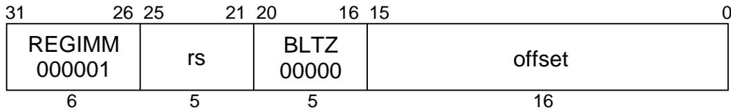
**MIPS I****Format:** BLTZ rs, offset**Purpose:** To test a GPR then do a PC-relative conditional branch.**Description:** if (rs < 0) then branch
