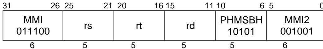
**C790****Format:** PHMSBH rd, rs, rt**Purpose:** To multiply 8 pairs of 16-bit signed integers and horizontally subtract.**Description:** (rd, HI, LO)  $\leftarrow$  rs  $\times$  rt – rs  $\times$  rt
