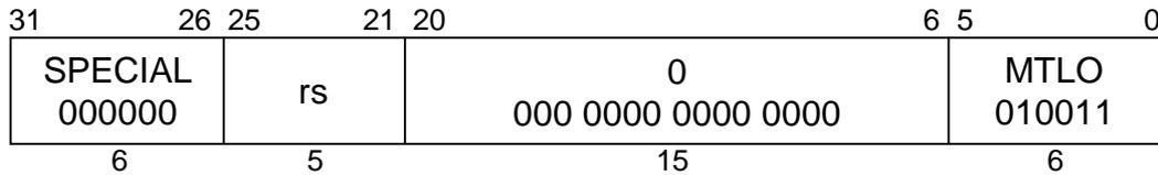
**MIPS I****Format:** MTLO rs**Purpose:** To copy a GPR to the special purpose LO register.**Description:**  $LO \leftarrow rs$
