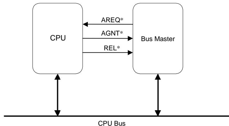
Figure 8-4. Connection of Arbitration Signals
