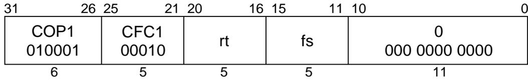
**MIPS I****Format:** CFC1 *rt*, *fs***Purpose:** To copy a word from an FPU control register to a GPR.**Description:**  $rt \leftarrow FP\_Control[fs]$
