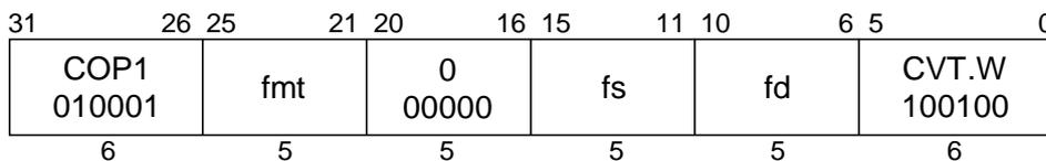
**MIPS I****Format:** CVT.W.S *fd*, *fs*CVT.W.D *fd*, *fs***Purpose:** To convert an FP value to a 32-bit fixed-point.**Description:**  $fd \leftarrow \text{convert\_and\_round}(fs)$
