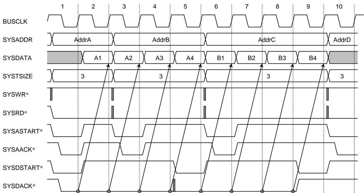
Figure 8-10. CPU Burst Reads
