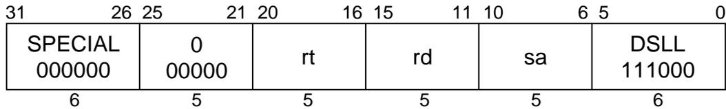
**MIPS III****Format:** DSLL rd, rt, sa**Purpose:** To left shift a doubleword by a fixed amount — 0 to 31 bits.**Description:**  $rd \leftarrow rt \ll sa$
