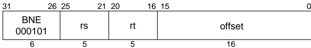
**MIPS I****Format:** BNE rs, rt, offset**Purpose:** To compare GPRs then do a PC-relative conditional branch.**Description:** if (rs  $\neq$  rt) then branch
