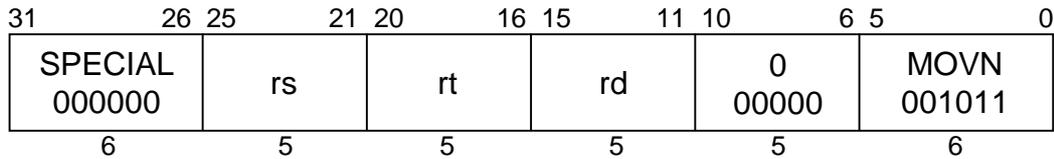
**MIPS IV****Format:** MOVN rd, rs, rt**Purpose:** To conditionally move a GPR after testing a GPR value.**Description:** if ( $rt \neq 0$ ) then  $rd \leftarrow rs$
