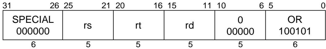
**MIPS I****Format:** OR rd, rs, rt**Purpose:** To do a bitwise logical OR.**Description:**  $rd \leftarrow rs \text{ OR } rt$
