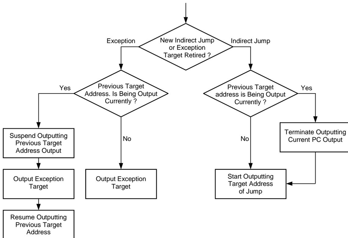
Figure 12-1. Priority of Outputting Jump or Exception Target
