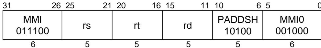
**C790****Format:** PADDSH rd, rs, rt**Purpose:** To add 8 pairs of 16-bit signed integers with saturation in parallel.**Description:**  $rd \leftarrow rs + rt$
