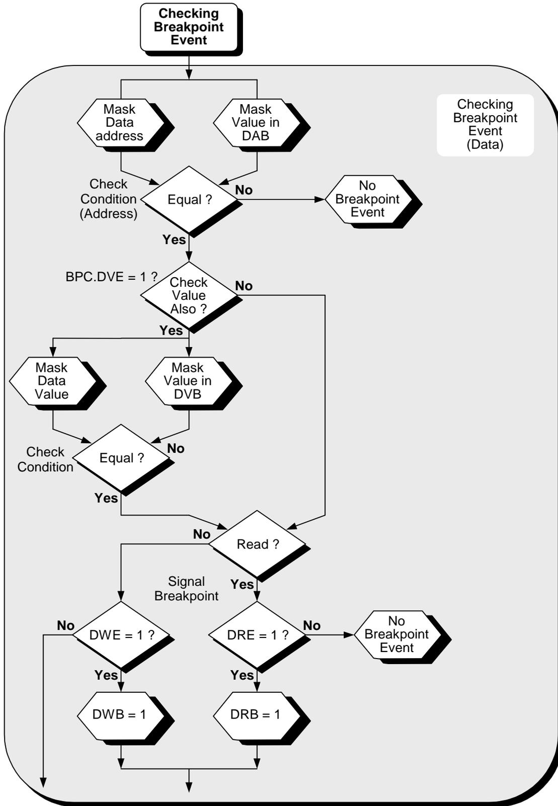
Figure 13-10. Hardware Breakpoint detection flow (DAB/DVB) (1/2)
