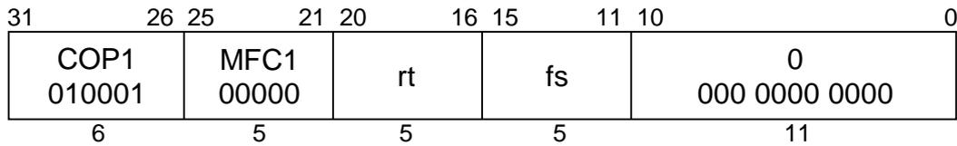
**MIPS I****Format:** MFC1 rt, fs**Purpose:** To copy a word from an FPU (COP1) general register to a GPR.**Description:**  $rt \leftarrow fs$
