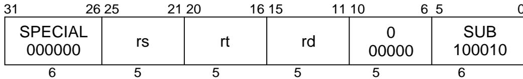
**MIPS I****Format:** SUB rd, rs, rt**Purpose:** To subtract 32-bit integers. If overflow occurs, then trap.**Description:**  $rd \leftarrow rs - rt$
