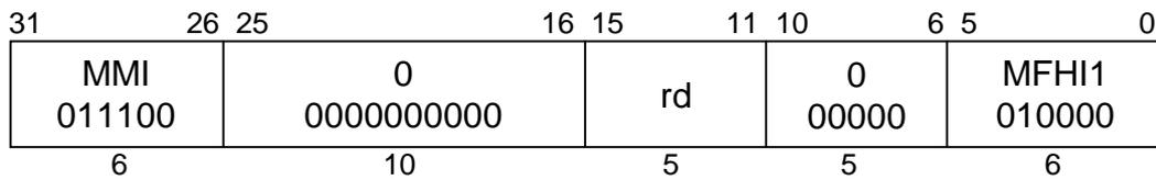
**C790****Format:** MFHI1 rd**Purpose:** To copy the special purpose register HI1 to a GPR.**Description:** rd ← HI1
