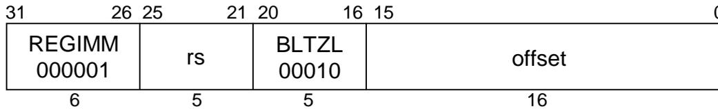
**MIPS II****Format:** BLTZL rs, offset**Purpose:** To test a GPR then do a PC-relative conditional branch; execute the delay slot only if the branch is taken.**Description:** if (rs < 0) then branch\_likely
