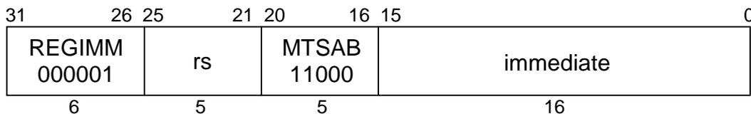
**C790****Format:** MTSAB rs, immediate**Purpose:** To copy a GPR to the shift amount register SA.**Description:**  $SA \leftarrow (rs \text{ xor } \text{immediate}) \times 8$
