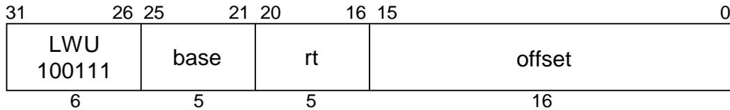
**MIPS III****Format:** LWU *rt*, *offset* (*base*)**Purpose:** To load a word from memory as an unsigned value.**Description:**  $rt \leftarrow \text{memory}[\text{base} + \text{offset}]$
