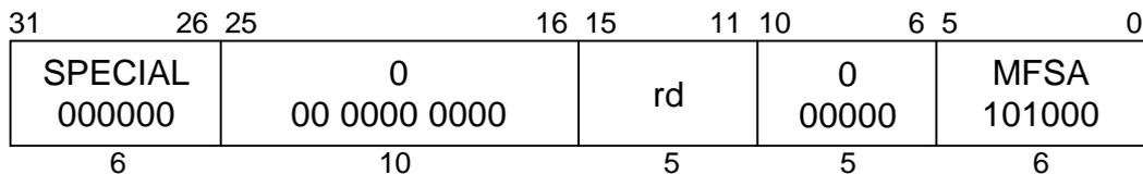
**C790****Format:** MFSA rd**Purpose:** To copy the shift amount register SA to a GPR.**Description:** rd ← SA
