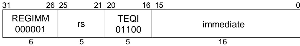
**MIPS II****Format:** TEQI rs, immediate**Purpose:** To compare a GPR to a constant and do a conditional Trap.**Description:** if (rs = immediate) then Trap
