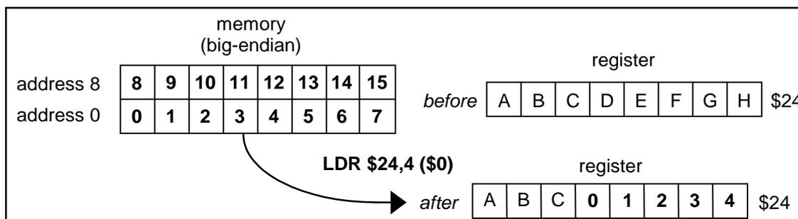
The contents of GPR *rt* are internally bypassed within the processor so that no NOP is needed between an immediately preceding load instruction which specifies register *rt* and a following LDR (or LDL) instruction which also specifies register *rt*.
