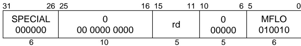
**MIPS I****Format:** MFLO rd**Purpose:** To copy the special purpose LO register to a GPR.**Description:** rd ← LO
