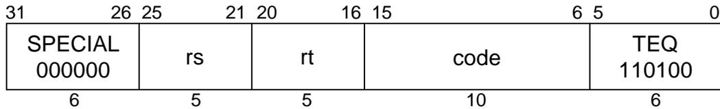
**MIPS II****Format:** TEQ rs, rt**Purpose:** To compare GPRs and do a conditional Trap.**Description:** if (rs = rt) then Trap
