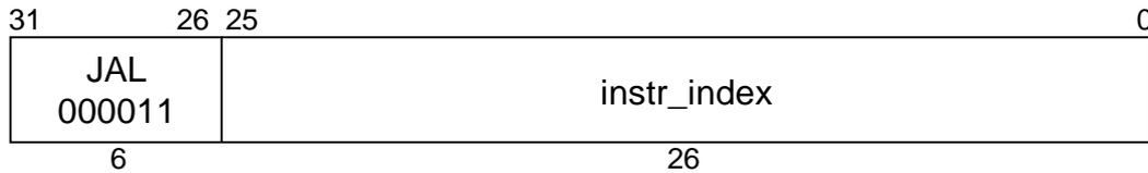
**MIPS I****Format:** JAL target**Purpose:** To procedure call within the current 256 MB aligned region.**Description:**
