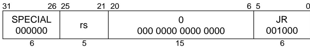
**MIPS I****Format:** JR rs**Purpose:** To branch to an instruction address in a register.**Description:** PC ← rs
