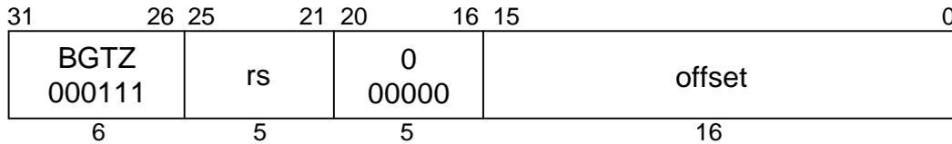
**MIPS I****Format:** BGTZ rs, offset**Purpose:** To test a GPR then do a PC-relative conditional branch.**Description:** if (rs > 0) then branch
