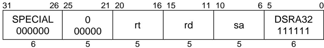
**MIPS III****Format:** DSRA32 rd, rt, sa**Purpose:** To arithmetic right shift a doubleword by a fixed amount — 32-63 bits.**Description:**  $rd \leftarrow rt \gg (sa + 32)$  (arithmetic)
