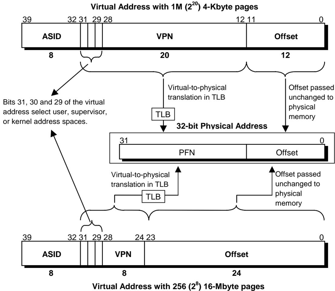
Figure 6-2. 32-bit Mode Virtual Address Translation
