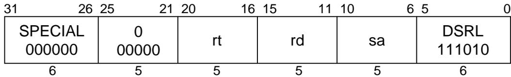
**MIPS III****Format:** DSRL rd, rt, sa**Purpose:** To logical right shift a doubleword by a fixed amount — 0 to 31 bits.**Description:**  $rd \leftarrow rt \gg sa$  (logical)
