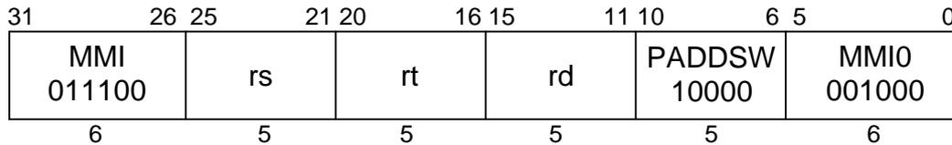
**C790****Format:** PADDSW rd, rs, rt**Purpose:** To add 4 pairs of 32-bit signed integers with saturation in parallel.**Description:**  $rd \leftarrow rs + rt$
