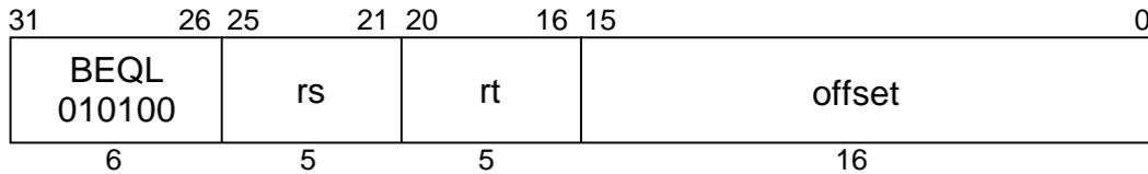
**MIPS II****Format:** BEQL rs, rt, offset**Purpose:** To compare GPRs then do a PC-relative conditional branch; execute the delay slot only if the branch is taken.**Description:** if (rs = rt) then branch\_likely
