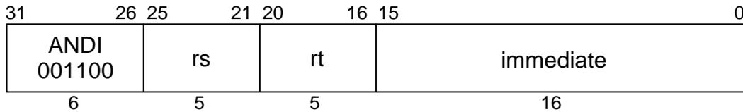
**MIPS I****Format:** ANDI *rt*, *rs*, *immediate***Purpose:** To do a bitwise logical AND with a constant.**Description:**  $rt \leftarrow rs \text{ AND } \textit{immediate}$
