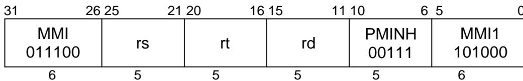
**C790****Format:** PMINH rd, rs, rt**Purpose:** To select the minimum of two 16-bit signed integers (8 parallel operations).**Description:**  $rd \leftarrow \min(rs, rt)$
