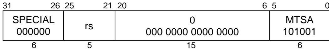
**C790****Format:** MTSA rs**Purpose:** To copy a GPR to the shift amount register SA.**Description:** SA ← rs
