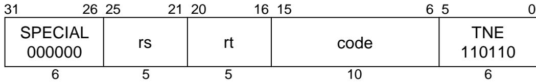
**MIPS II****Format:** TNE rs, rt**Purpose:** To compare GPRs and do a conditional Trap.**Description:** if ( $rs \neq rt$ ) then Trap
