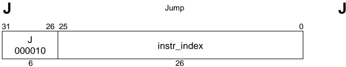
**MIPS I****Format:** J target**Purpose:** To branch within the current 256 MB aligned region.**Description:**
