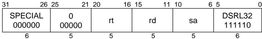
**MIPS III****Format:** DSRL32 rd, rt, sa**Purpose:** To logical right shift a doubleword by a fixed amount — 32 to 63 bits.**Description:**  $rd \leftarrow rt \gg (sa + 32)$  (logical)
