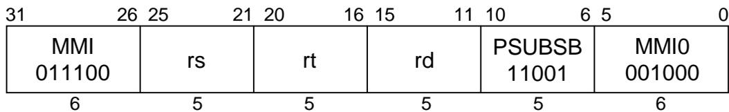
**C790****Format:** PSUBSB rd, rs, rt**Purpose:** To subtract 16 pairs of 8-bit signed integers with saturation in parallel.**Description:**  $rd \leftarrow rs - rt$
