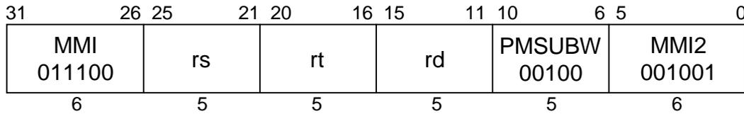
**C790****Format:** PMSUBW rd, rs, rt**Purpose:** To multiply 2 pairs of 32-bit signed integers and subtract in parallel.**Description:** (rd, HI, LO) ← (HI, LO) – rs × rt
