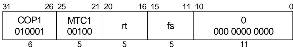
**MIPS I****Format:** MTC1 rt, fs**Purpose:** To copy a word from a GPR to an FPU (COP1) general register.**Description:** fs ← rt
