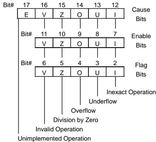
Figure 10-4. Control/Status Register Cause, Flag, and Enable Fields
