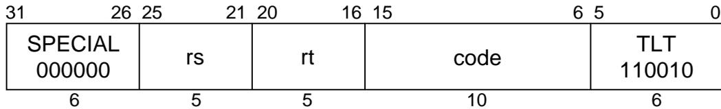
**MIPS II****Format:** TLT rs, rt**Purpose:** To compare GPRs and do a conditional Trap.**Description:** if (rs < rt) then Trap
