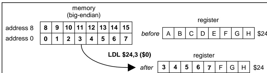
The contents of GPR *rt* are internally bypassed within the processor so that no NOP is needed between an immediately preceding load instruction which specifies register *rt* and a following LDL (or LDR) instruction which also specifies register *rt*.
