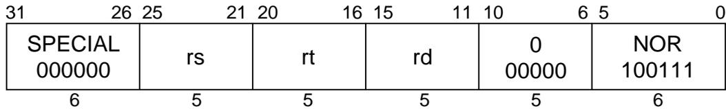
**MIPS I****Format:** NOR rd, rs, rt**Purpose:** To do a bitwise logical NOT OR.**Description:**  $rd \leftarrow rs \text{ NOR } rt$
