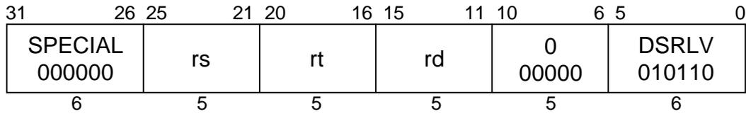
**MIPS III****Format:** DSRLV rd, rt, rs**Purpose:** To logical right shift a doubleword by a variable number of bits.**Description:**  $rd \leftarrow rt \gg rs$  (logical)
