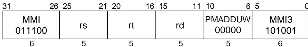
**C790****Format:** PMADDUW rd, rs, rt**Purpose:** To multiply 2 pairs of 32-bit unsigned integers and accumulate in parallel.**Description:** (rd, HI, LO) ← (HI, LO) + rs × rt
