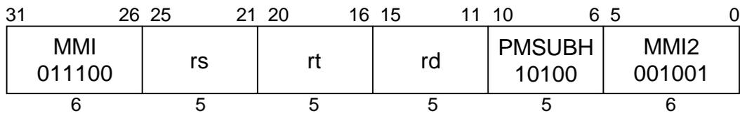
**C790****Format:** PMSUBH rd, rs, rt**Purpose:** To multiply 8 pairs of 16-bit signed integers and subtract in parallel.**Description:** (rd, HI, LO) ← (HI, LO) – rs × rt
