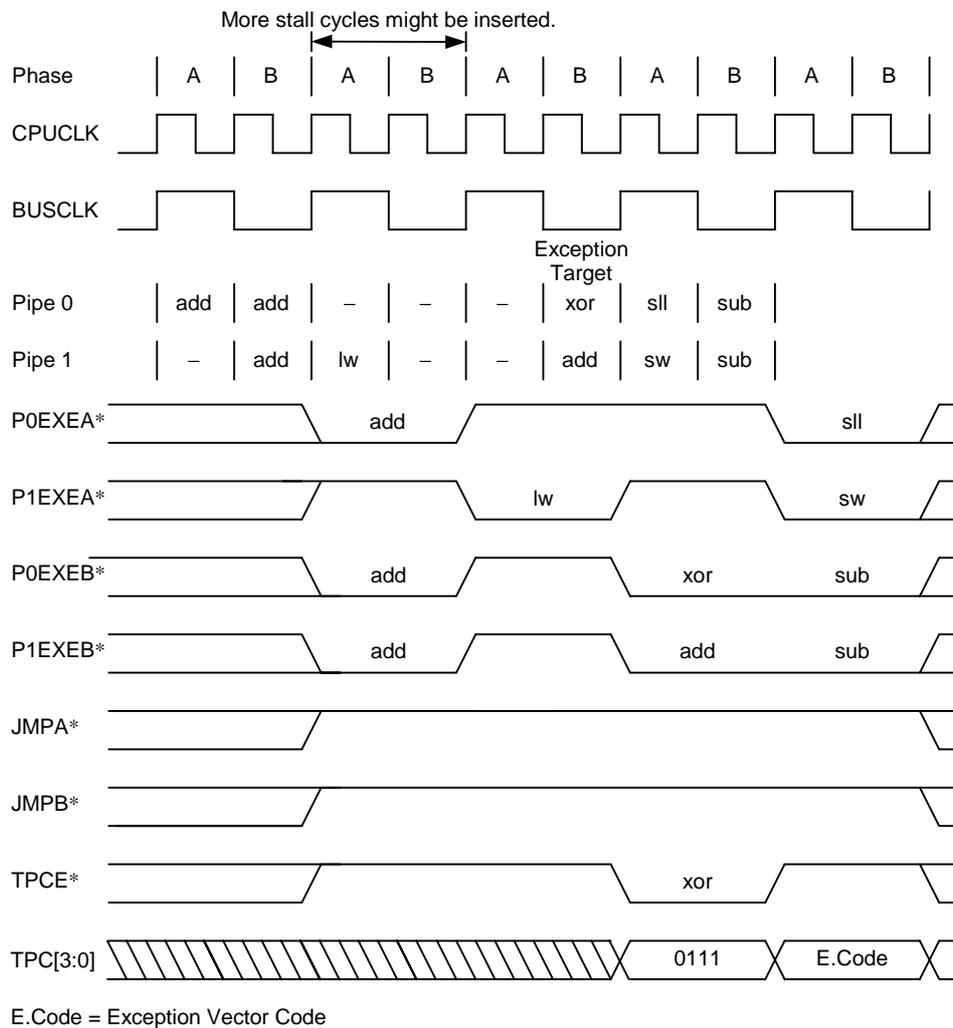
Figure 12-7. Waveform for Exception (Target in Phase B)
