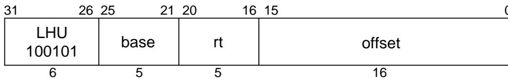
**MIPS I****Format:** LHU *rt*, *offset* (*base*)**Purpose:** To load a halfword from memory as an unsigned value.**Description:**  $rt \leftarrow \text{memory}[\text{base} + \text{offset}]$
