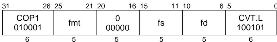
**MIPS III****Format:** CVT.L.S *fd*, *fs*CVT.L.D *fd*, *fs***Purpose:** To convert an FP value to a 64-bit fixed-point.**Description:**  $fd \leftarrow \text{convert\_and\_round}(fs)$
