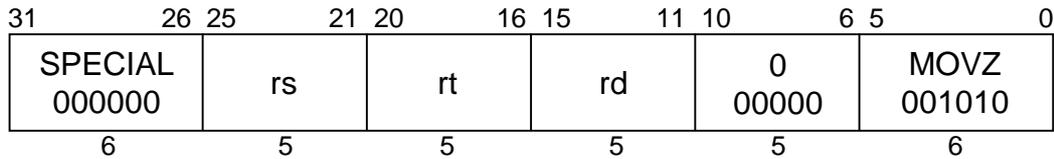
**MIPS IV****Format:** MOVZ rd, rs, rt**Purpose:** To conditionally move a GPR after testing a GPR value.**Description:** if (rt = 0) then rd ← rs
