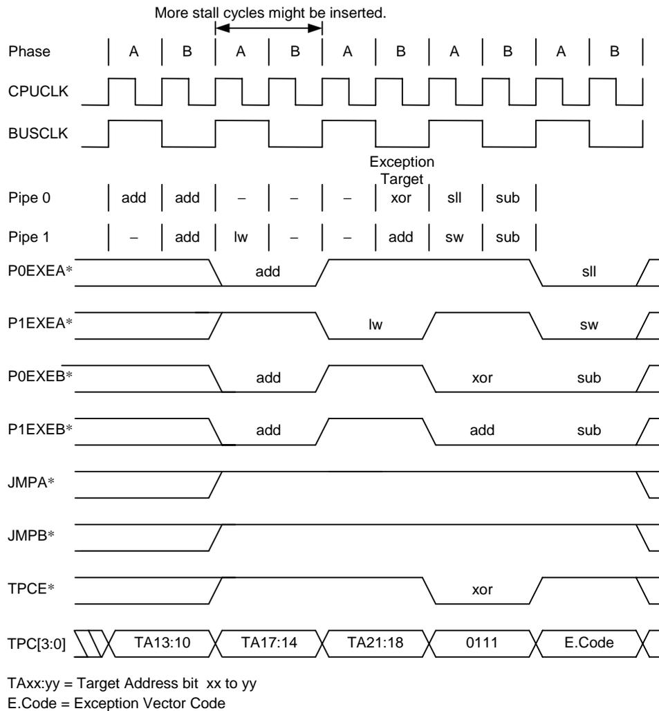
Figure 12-8. Waveform for Exception (During Target PC Output)
