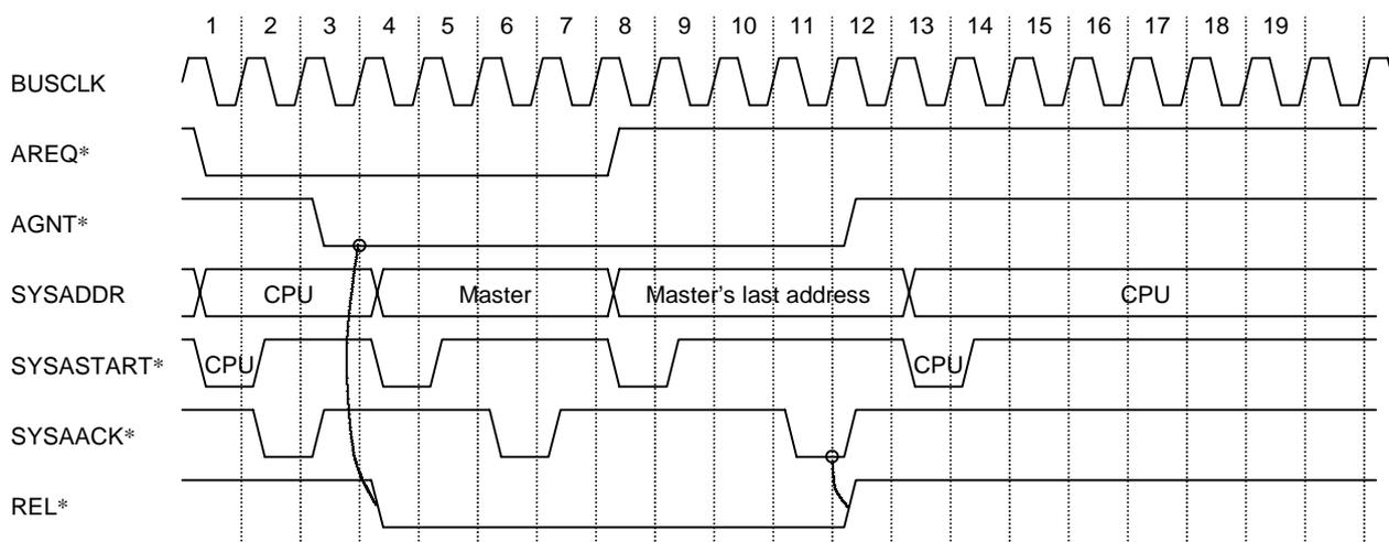
Figure 8-6. Cycle Stealing Protocol
