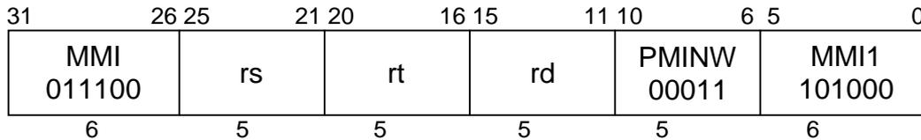
**C790****Format:** PMINW rd, rs, rt**Purpose:** To select the minimum of two 32-bit signed integers (4 parallel operations).**Description:**  $rd \leftarrow \min(rs, rt)$
