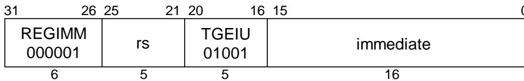
**MIPS II****Format:** TGEIU rs, immediate**Purpose:** To compare a GPR to a constant and do a conditional Trap.**Description:** if ( $rs \geq \text{immediate}$ ) then Trap
