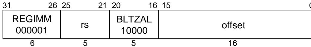
**MIPS I****Format:** BLTZAL rs, offset**Purpose:** To test a GPR then do a PC-relative conditional procedure call.**Description:** if (rs < 0) then procedure\_call
