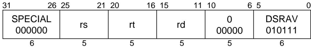
**MIPS III****Format:** DSRAV rd, rt, rs**Purpose:** To arithmetic right shift a doubleword by a variable number of bits.**Description:**  $rd \leftarrow rt \gg rs$  (arithmetic)
