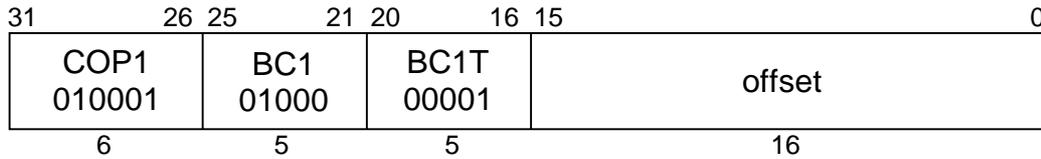
**MIPS I****Format:** BC1T offset**Purpose:** To test an FP condition code and do a PC-relative conditional branch.**Description:** if (C = 1) then branch where C is FCR31<sub>23</sub>.
