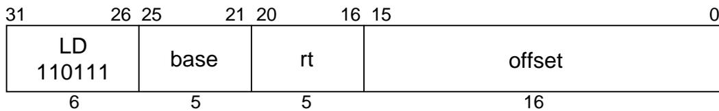
**MIPS III****Format:** LD *rt*, *offset* (*base*)**Purpose:** To load a doubleword from memory.**Description:**  $rt \leftarrow \text{memory}[\text{base} + \text{offset}]$
