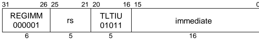
**MIPS II****Format:** TLTIU rs, immediate**Purpose:** To compare a GPR to a constant and do a conditional Trap.**Description:** if (rs < immediate) then Trap
