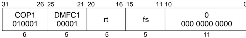
**MIPS III****Format:** DMFC1 rt, fs**Purpose:** To copy a doubleword from an FPR to a GPR.**Description:**  $rt \leftarrow fs$
