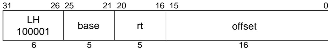
**MIPS I****Format:** LH *rt*, *offset* (*base*)**Purpose:** To load a halfword from memory as a signed value.**Description:**  $rt \leftarrow \text{memory}[\text{base} + \text{offset}]$
