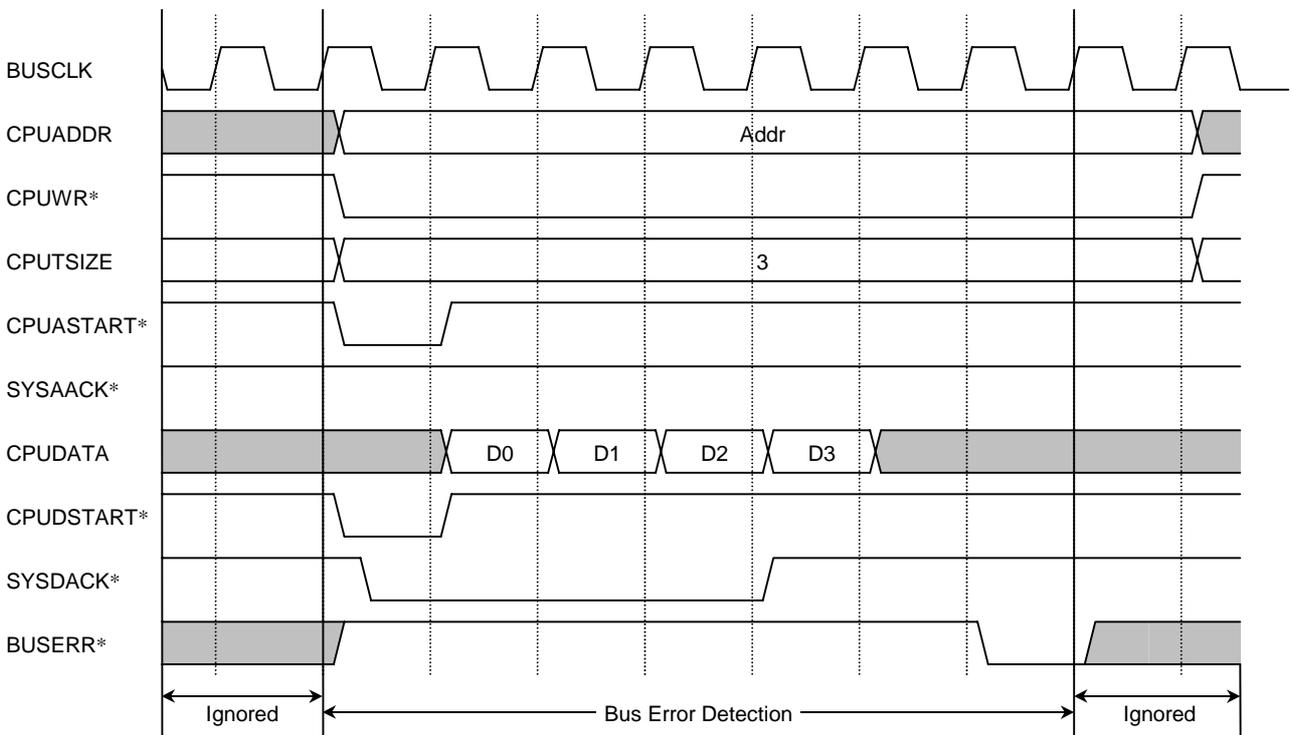
Figure 8-19. One Operation with BUSERR\* as SYSAACK\*
