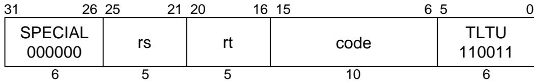
**MIPS II****Format:** TLTU rs, rt**Purpose:** To compare GPRs and do a conditional Trap.**Description:** if (rs < rt) then Trap
