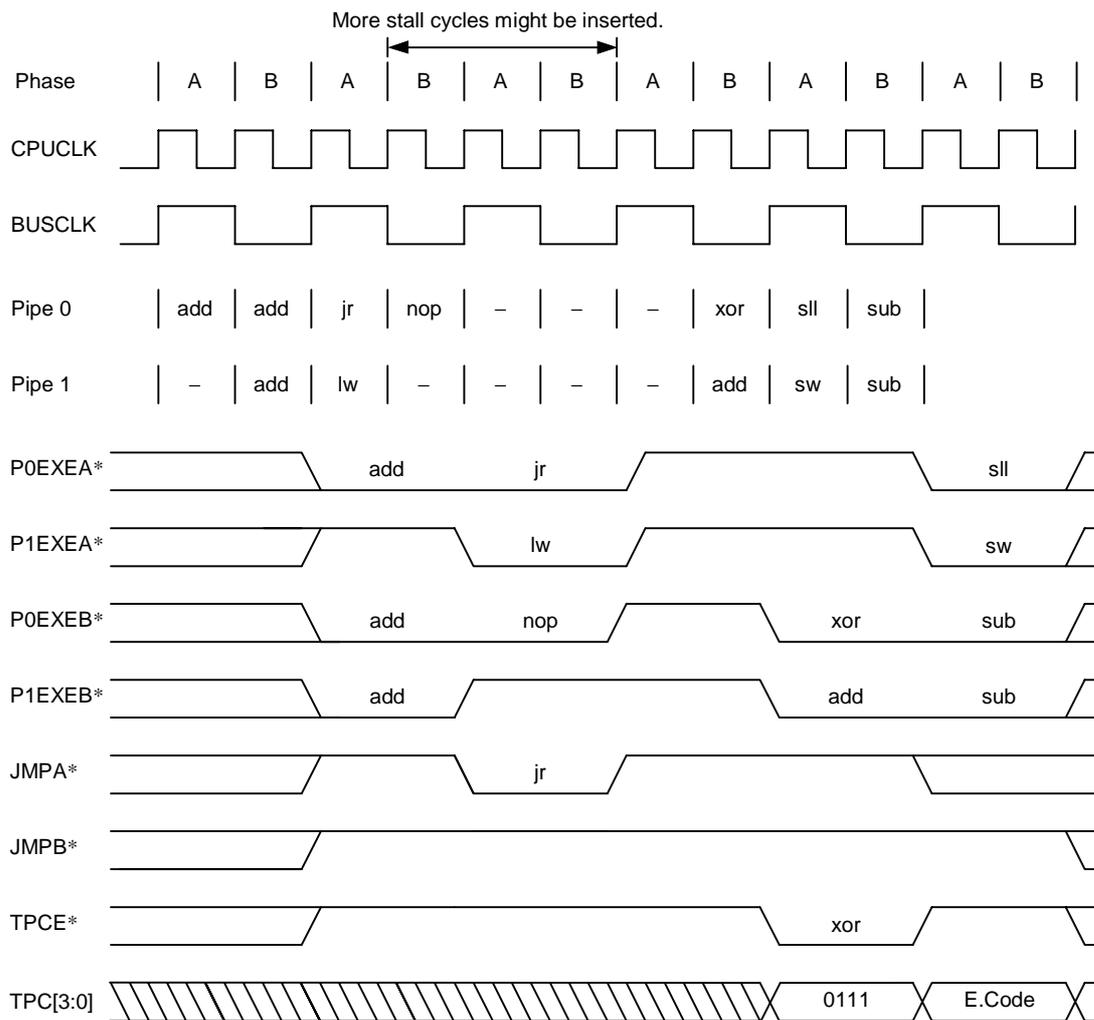
Figure 12-11. Waveform for Exception Generated by Target Instruction
