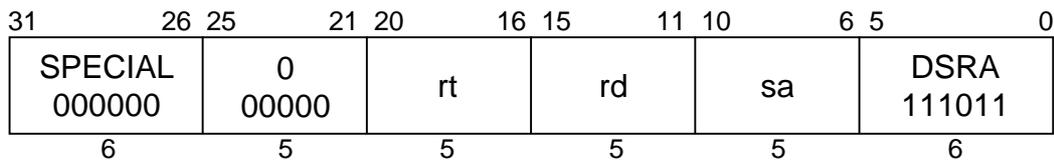
**MIPS III****Format:** DSRA rd, rt, sa**Purpose:** To arithmetic right shift a doubleword by a fixed amount — 0 to 31 bits.**Description:**  $rd \leftarrow rt \gg sa$  (arithmetic)
