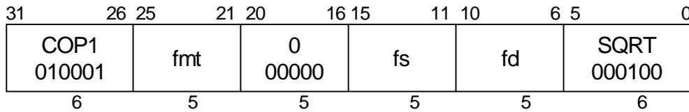
**MIPS II****Format:** SQRT.S *fd*, *fs*SQRT.D *fd*, *fs***Purpose:** To compute the square root of an FP value.**Description:**  $fd \leftarrow \text{SQRT}(fs)$
